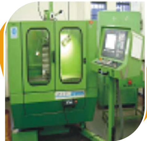
WF3 1D1 Mikron Travel Size : X=450, Y=400, Z=400
