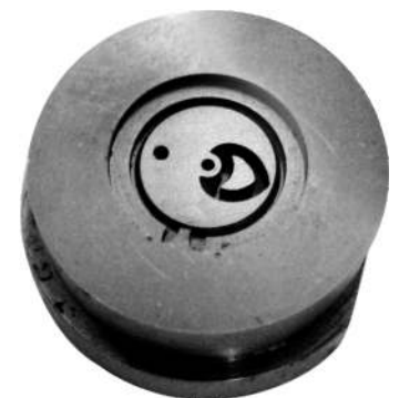
Cavity Insert with high finish
