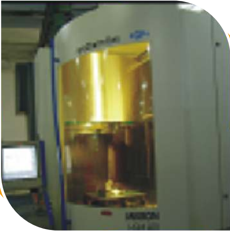
High Speed HSM600 Mikron Travel Size : X=600, Y=600, Z=450
