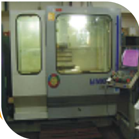
5 Axis UM710 Mikron Travel Size : X=710, Y=630, Z=500
