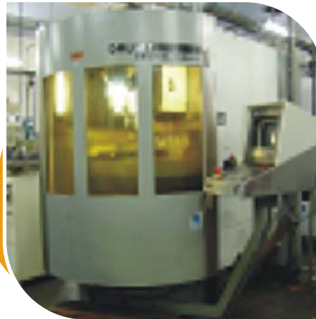
DMU60T Deckel Maho Travel Size : X=630, Y=560, Z=560
